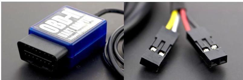
Figura 31 : UART Adapter per CanBus Sniffer
